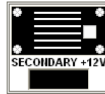
FIGURE 22: ICON POWER SUPPLY WITH CONTINUOUS CURRENT, SECONDARY POSITION.
